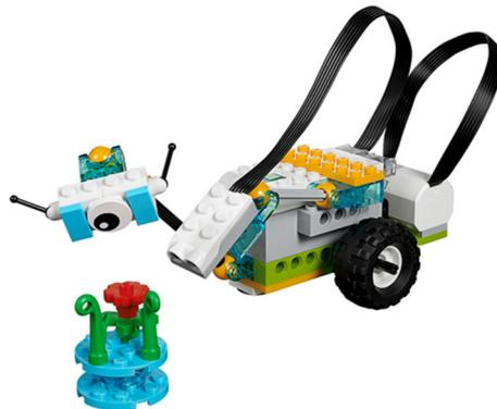
The team must use the mobile WeDo car to demonstrate what autonomous emergency braking is. The mobile WeDo car must be programmed to autonomously drive forward until the motion sensor mounted on the car detects an object in front of the car. When an object is detected, the car must stop. The autonomously driven car must be controlled by a sequence of WeDo commands that, once activated, make the car drive on its own, i.e. the car must not be remotely controlled.
